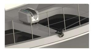
The deck mount sensor can be used if the deck is higher than the railing or there is a point to mout the line sensor in front of the railing.
